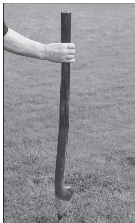
Photo 4 A potato dibber or stíbhín with a forged steel tip
